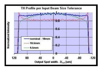
\*\*Interesting to note in fig.6, that this gives a very similar effect as in fig.5. There is a clear parallel between too large beam size and extended defocus. The "dog ears" effect is the same.
