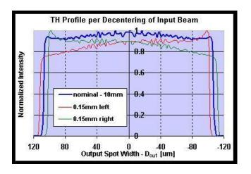
Fig. 4: Effect of x-axis or y-axis de-centering of input beam on Top-Hat Profile
