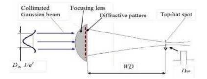
The diffractive beam shaper is a phase element that transforms the Gaussian input beam into a uniform spot with sharp edges at a specific working distance WD.
