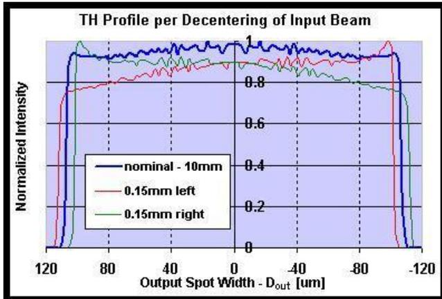
\*\*Noteworthy in figure 4 above is the "tilted" Top-Hat profile due to de-centering; i.e. a slope in the intensity going from one side of the spot to the other.
