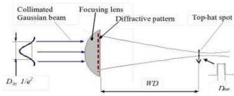
The diffractive beam shaper is a phase element that transforms the Gaussian input beam into a uniform spot with sharp edges at a specific working distance WD.
