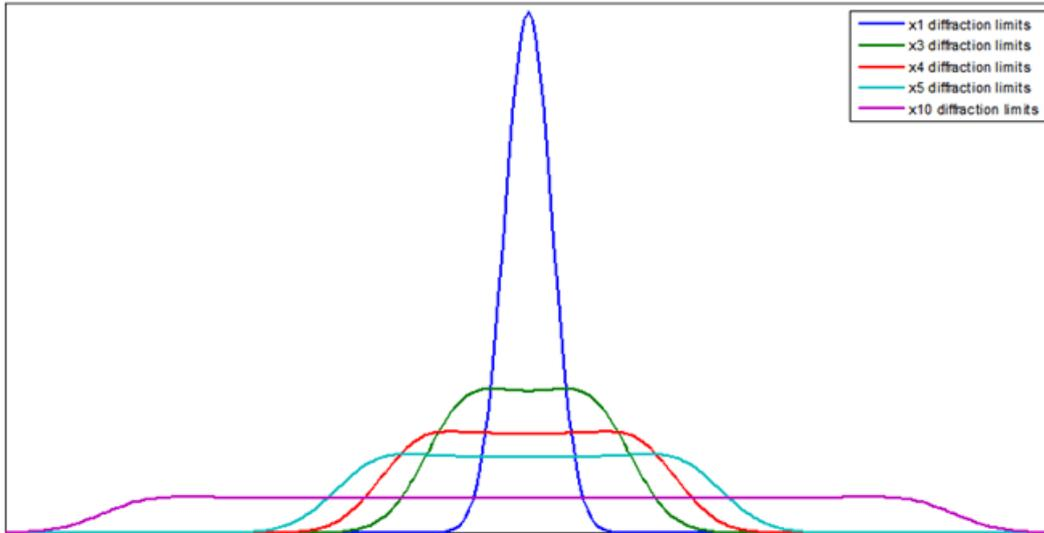
A typical application prefers the transfer region (13.5-90 %) to be as small as possible and the Top Hat profile to have a maximum relative size of uniform area.
