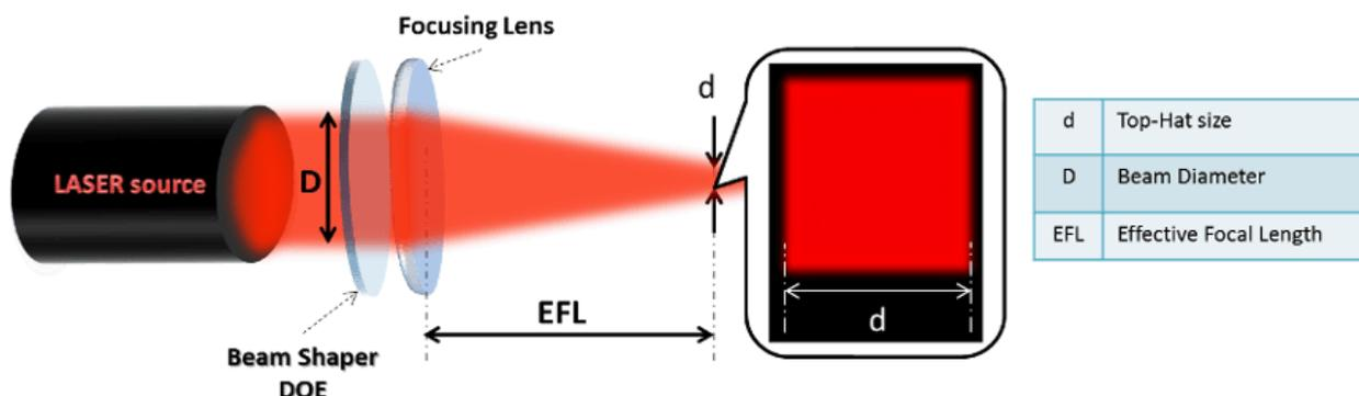
The advantage of working with a larger input beam is twofold. First, a larger beam reduces somewhat the sensitivity of the beam shaper output to tolerances. Secondly, a larger input beam will enable achieving a smaller output spot, which is a desired outcome for many beam shapers applications.
